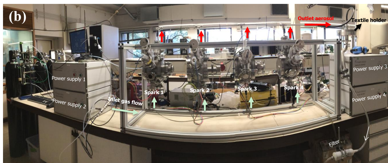
Figure S7.6. Schematic illustration (a) and the photograph (b) of the experimental setups for textile nanofinishing using four spark ablation systems for producing the NPs. Key: MPS: mini-particle sampler; DMA: differential mobility analyzer; AEM: aerosol electrometer.
