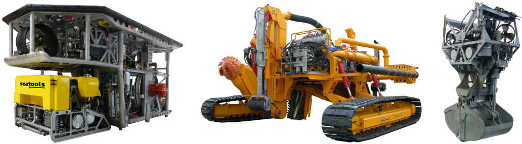
Figure 1.1: Selection of developed remotely operated vehicles by Seatools BV. On the left a rock-dump ROV Rockpiper depicted with integrated survey ROV which can undock from the main ROV. In the middle is a trencher Arthropod 600 depicted which can bury pipes up to 1.2 m in diameter. On the right is a grab excavation system GES depicted, which can collect or remove sand or clay material from the seabed. All figures above are shown with the courtesy of Seatools BV.
