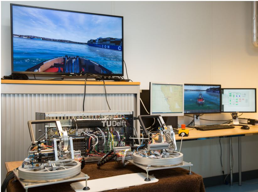
Figure A.12: Gemini Mark II maritime simulator, including a high-end tugboat simulation NAUTIS, using VSTEP Simulation.
