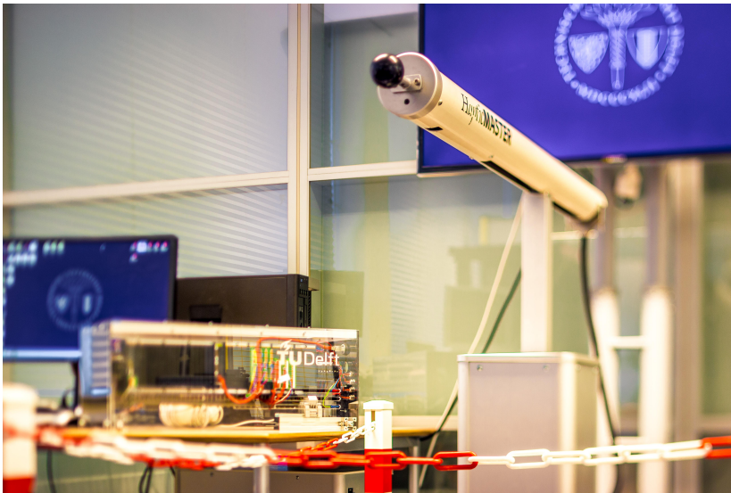
Figure A.5: HapticMASTER setup including Bachmann controller, capable of a four-channel controller for position and rate controlled tasks.
