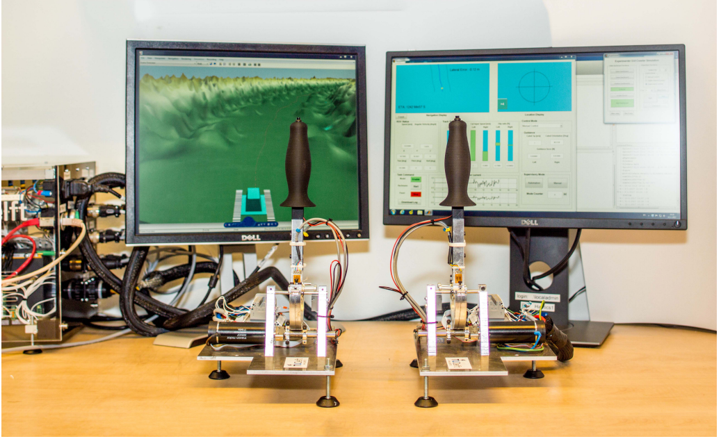
Figure 8.1: Overview of the developed experimental setup Gemini, consisting of two 1 DOF control input handles with force feedback capability. Behind the input handles two displays show the 3D modeled virtual environment (left screen), and the control panel with relevant information about the crawler (e.g. track speeds, water current and vehicle status), as well as a display for a secondary task.
