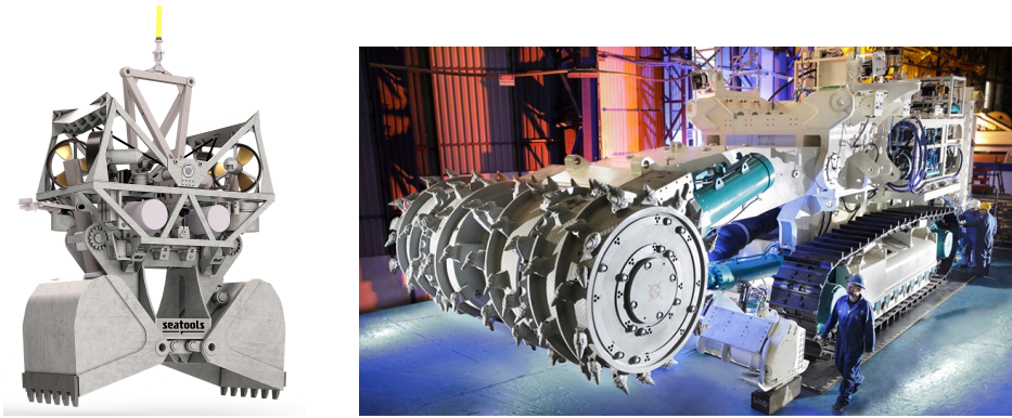
Figure 1.3: Deep-sea mining machines. On the left is a proposed deep-sea mining grab of Seatools BV depicted. On the right is a drum-cutter of Nautulus Minerals depicted, developed for deep-sea mining at the Solwara-1 project in Papua New Guinea. Both figure above are shown with the courtesy of Seatools BV and Nautulus Minerals
