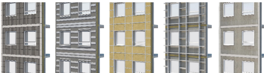
Figure 3: Renderings of the new façade construction. From right to left; original concrete tile façade, new steel rafters attached to the original façade, insulation, windstop and rafters, new concrete tiles. Renderings by JJW Architects.
