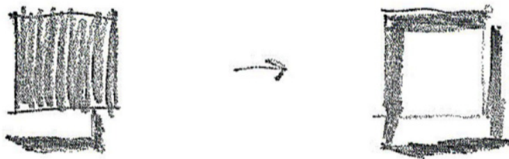
Figure 2: Sketch made by JJW Architects showing the shadow effect of an original, recessed, open balcony with flower bowl and the expected visual effect of the future solution with the slightly recessed glass covering and the new concrete box.
