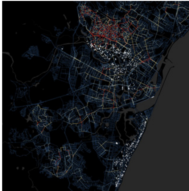
Figure 8 - Local angular choice with the location of towers on podium (in white) Source: Author's own.
