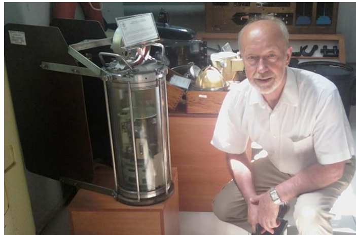
Fig. 2 Strong cylindrical shell of underwater oceanographic device made of glass tube.
