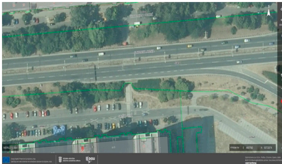
Figure 12. Pedestrian passage under the street in Zagreb, Savica, on the State Geodetic Administration Geoportal (digital ortophoto image overlapped with digital cadastral map) [37].
