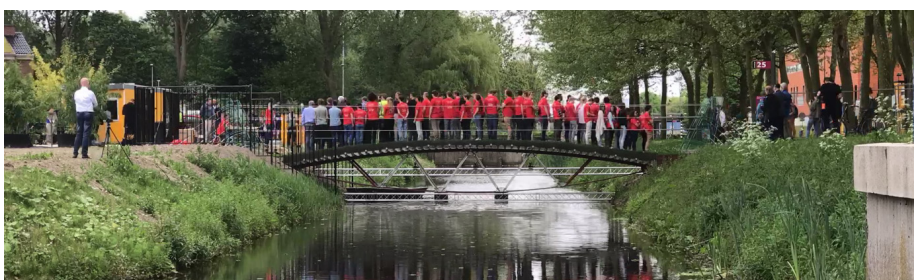
Figure 28 : Load case 1, 67 students, approximately 1.81 kN/m
