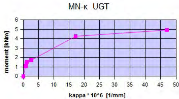
Figure 6: MN- \kappa diagram, ultimate state for a normal force N_d = 44,8 kN.
