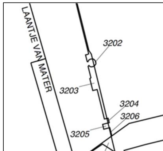
Figure 12. Tiny parcels due to the division of ground parcels in the Delft case to permit the 2D map to reflect objects above and below the surface.
