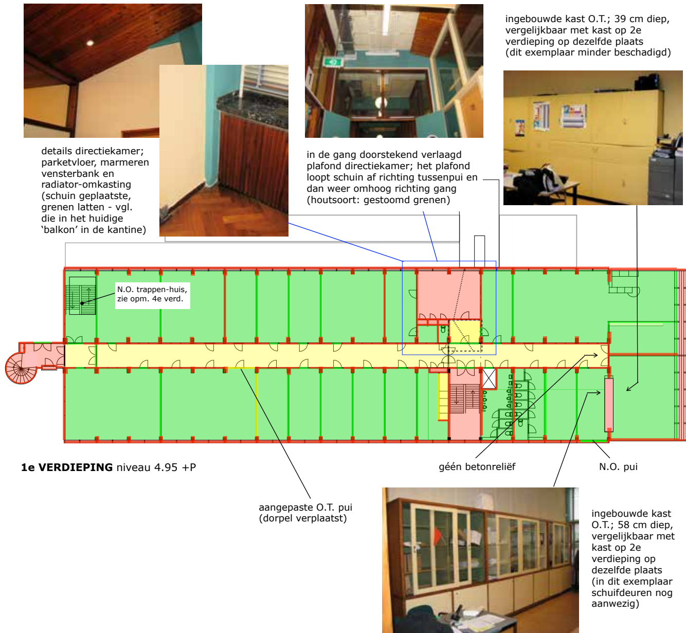
FIG. 5.12 The floor plan of the Patrimonium Technical School reworked into a historical atlas for the Historic Building Survey Report in 2011, indicating various levels of cultural historic value: high (red), limited (amber) and indifferent (green) / Suzanne Fischer
