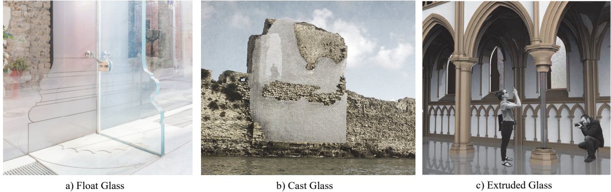
Fig. 11 a) Abstract interpretation of Corinthian style column using float glass fins (Gnosis Architettura and Bardeschi 2017), b) Glass masonry that consists of interlocking cast glass units (Barou 2016) and c) Restoration of Gothic columns with extruded glass tubes (Van den Broek 2017).
