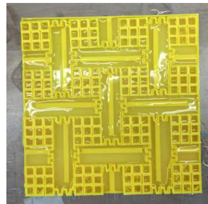
Figure 5. Cast of ABS matrices into shallow silicone sheets.
