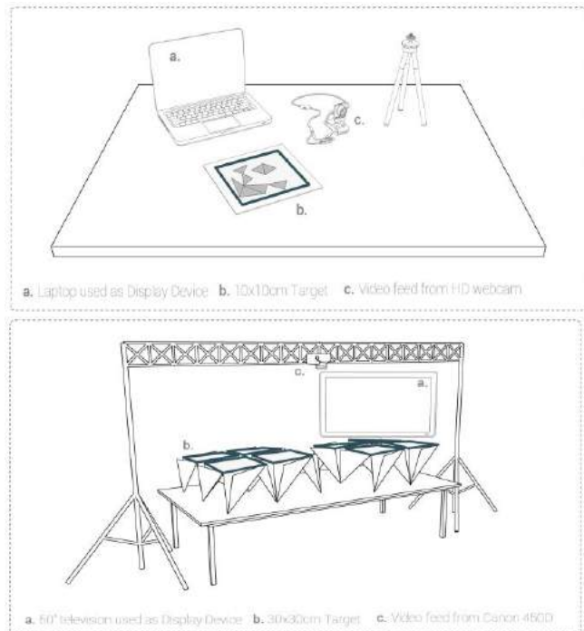
Figure 5. Experiment setup for a 100x120cm test (top) and a 200x200cm test area (bottom).
