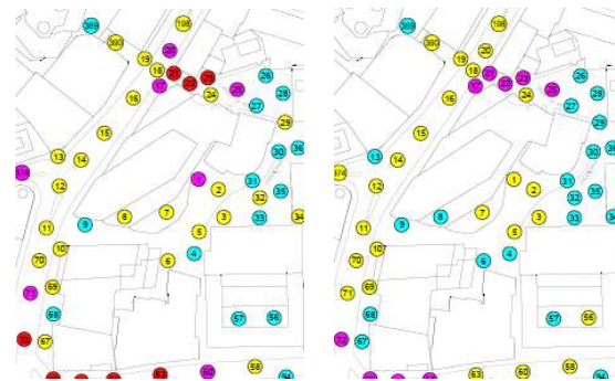
Figure 8. Wind tunnel results around the Eastern Cluster (New York meteorological data on the left, Toronto meteorological data on the right)
