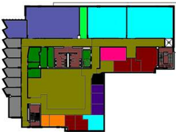
Figure 4. Thermal Zoning outcome from a previously developed algorithm showing unrealistic grouping of north and south rooms into a single zone.
