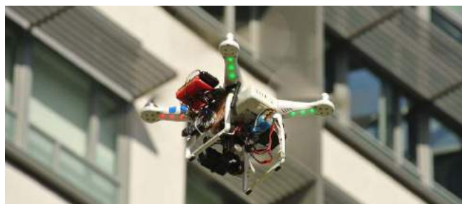
Figure 2, 3. UAV carrying gyro-stabilized GoPro and sensors, APM and GPS.
