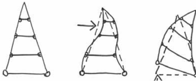
FIG. 12 Sketch of Movement of the Fin-Ray Effect
