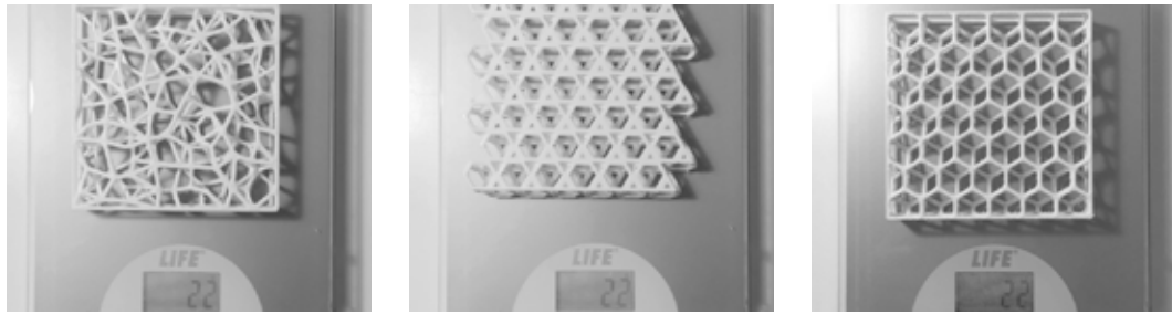
FIG. 2 Left: Undirected Vornoi Middle: Directed Vornoi Right: Kangome Structure
