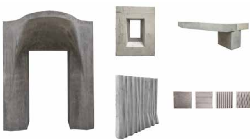
FIG. 7 ILC prototypes: façade element (2.5m(W)x3.0m(H)), window detail (1m(W)x1.25(H)), ILC balcony with normal concrete slab (2.5m(W)x0.97m(H)x0.8m(D)), surface designs (2.0m(W)x1.8m(H)) and samples 0.5m x 0.5m (Leibinger et al. 2016)
