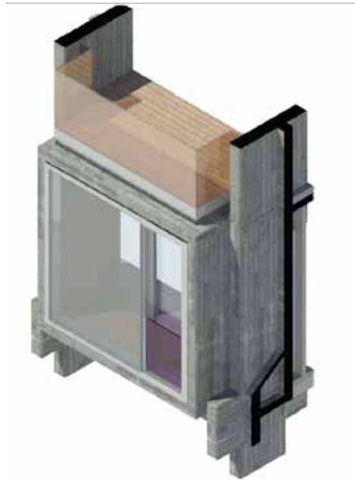
FIG. 6 To further emphasize the image of the all-glass effect at the corners or the openings, the outer slab of the insulating glazing extends 10-15 cm beyond the inner slab to cover the rising.
