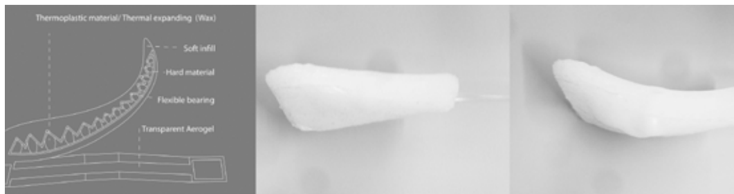
FIG. 11 Left: Section of volume chamber, Middle and Right: Model with integrated volume chamber to specify the movement with a thermodynamic material
