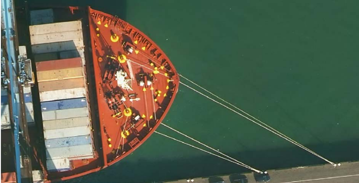
Figure 4. Mooring lines at forecastle deck in Rotterdam (photo Port of Rotterdam)
