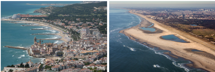
Fig. 6: Engineered shoreline with breakwaters and groins (Sitges, Spanje, left) en Pilot Sand Motor Delfland dd. February 16, 2016 (right)
