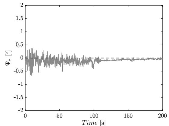
Fig. 17 Performance of the kite attitude controller.
