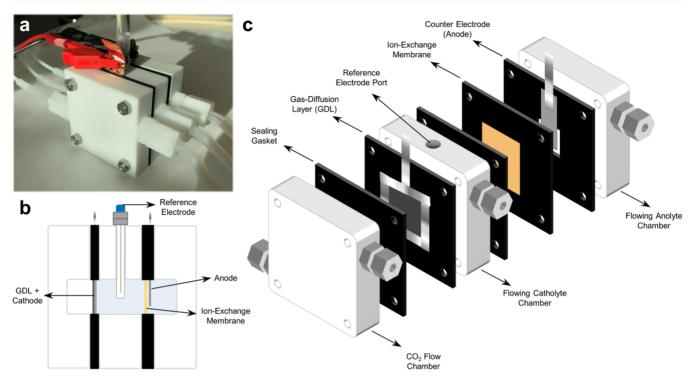
Figure 1. (a) A standard electrochemical for CO<sub>2</sub> electrolysis for testing catalysts in a three-electrode configuration. (b) Side profile showing chambers for the CO<sub>2</sub> (left), catholyte (center), and anolyte (right). (c) Isometric view of the exploded three-chamber cell showing individual components.
