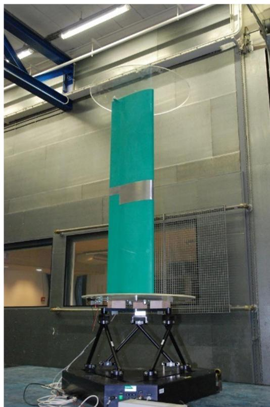
Fig. 2 The wing model on the 6-DOF platform.
