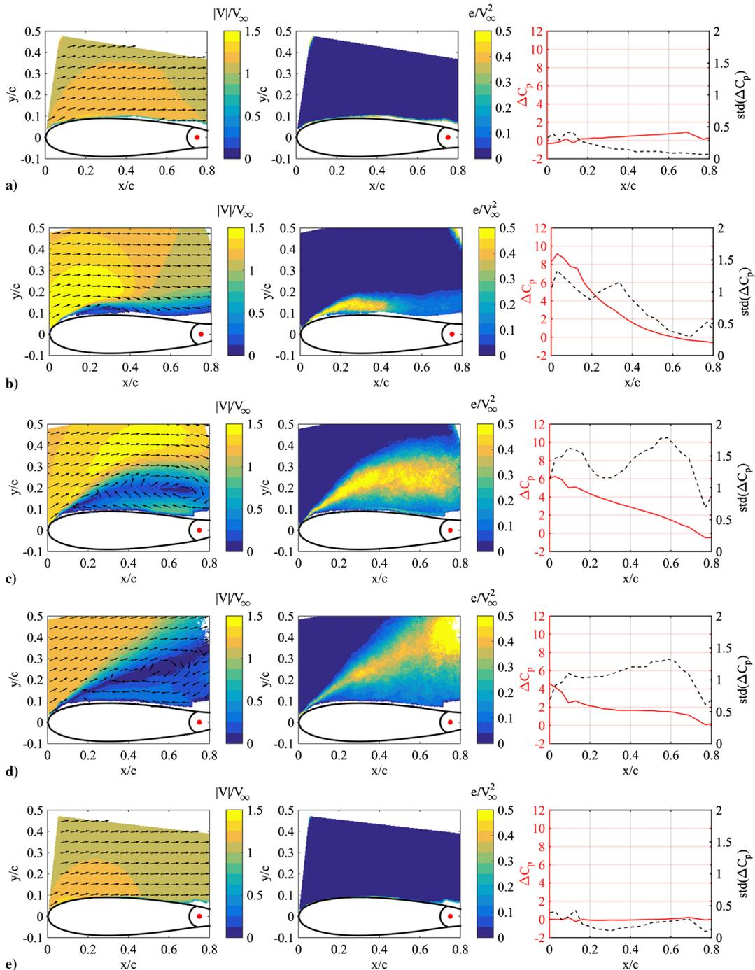
**Fig. 9** Left) Velocity magnitude contour plots with superposed vector arrows. Center) Turbulent kinetic energy contour plots. Right) Phase-averaged mean and standard deviation of differential pressure coefficient. a)–e) Refers to selected time instants as in Fig. 8.
