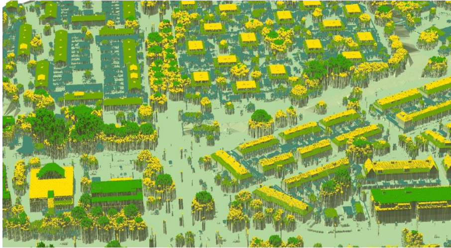
Figure 3. 'Model 1' digital surface model produced with first return points of AHN3
