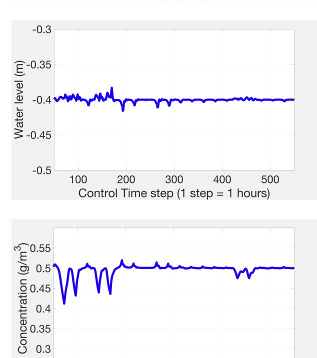
ii) Flushing with MPC
