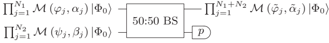
FIG. 3. Single round of a breeding protocol. The round takes approximate grid states defined by N_1 and N_2 measurement operators \mathcal{M} as inputs. It returns an approximate grid state with N_1 + N_2 (possibly changed) measurement operators. The second output port is subject to a homodyne measurement of the \hat{p} quadrature. The initial state |\Phi_0\rangle is chosen to be invariant under the action of a beam splitter, e.g., a squeezed vacuum state.
