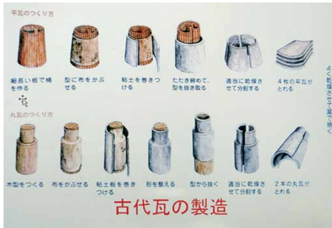
FIG. 17 Tile production in the past, with two pieces folded round a mould
