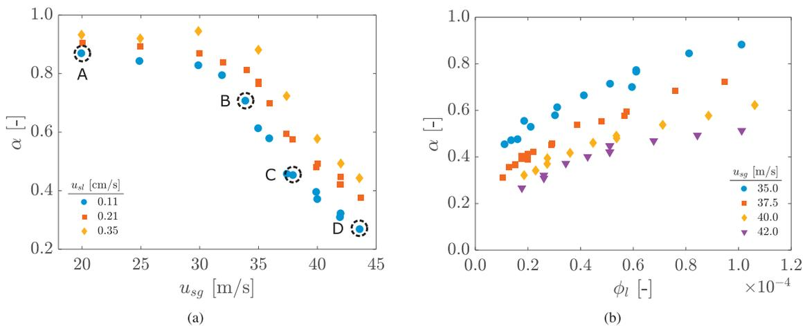
**Fig. 19.** Cavity filling as a function of the superficial gas speed  $u_{sg}$  (a) and the liquid volume fraction  $\phi_l$  (b). A–D in (a) correspond to the respective filling contours displayed in Fig. 20.
