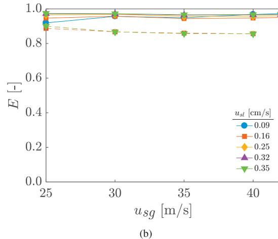
**Fig. 22.** Liquid entrainment as a function of the superficial gas velocity in a corrugated pipe, for different liquid loadings. Pipe with geometry A (a) and geometry B (b). Solid lines are for water, dashed lines for MEG. Results for water injection in geometry A are depicted in Fig. 17(b).
