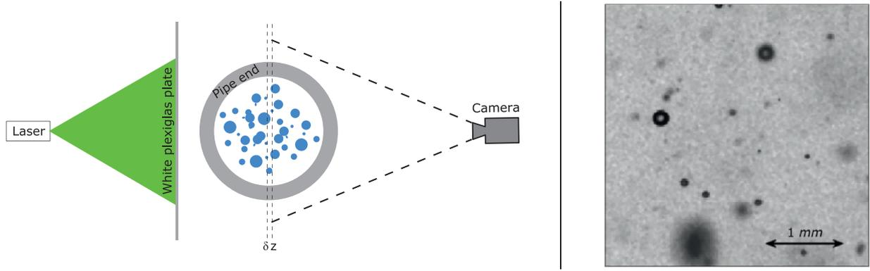
**Fig. 9.** Schematic representation of the shadowgraphy set-up (left), where  $\delta z$  depicts the depth of focus of the imaging system. A cut-out of a typical image obtained using the shadowgraphic measurement technique (right), after background subtraction and the application of a median filter. Dark spots are the shadows of droplets, used to find the droplet size.
