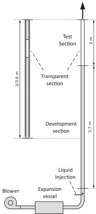
**Fig. 3.** Schematic representation of the experimental set-up. The gas flow is created using a blower, followed by an expansion vessel which reduces the noise amplitude from the blower. Liquid is injected with a spray nozzle at the pipe center. The test section is transparent and can be replaced by a corrugated pipe section.
