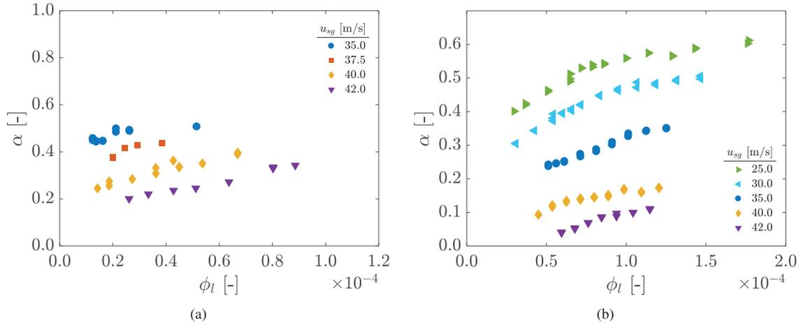
**Fig. 23.** Cavity filling as a function of liquid volume fraction  $\phi_l$ , for different superficial gas flow speeds. (a) Filling for MEG injection in geometry A, and (b) for water injection in geometry B.
