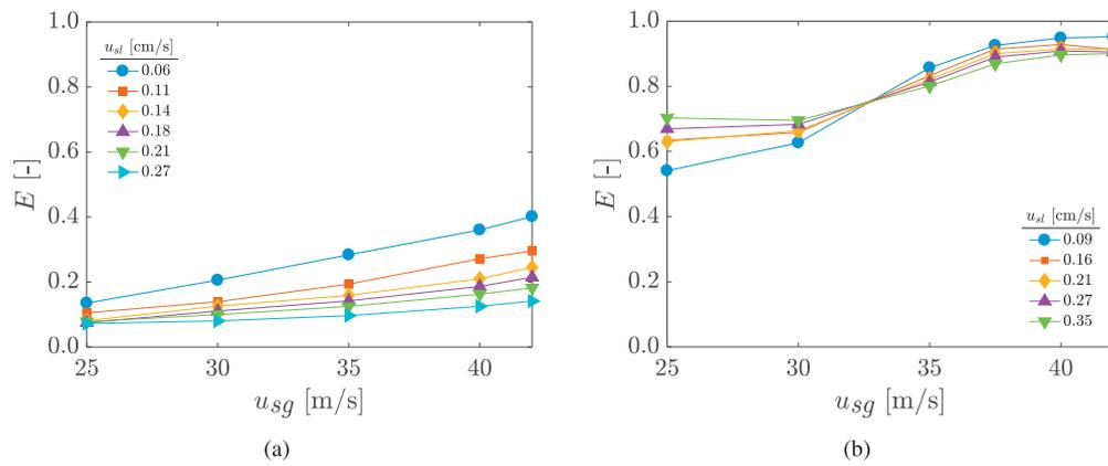
**Fig. 17.** Liquid entrainment ratio as a function of the superficial gas velocity  $u_{sg}$  for different values of the superficial liquid velocity  $u_{sl}$ , in smooth (a) and corrugated pipes (b, geom A).
