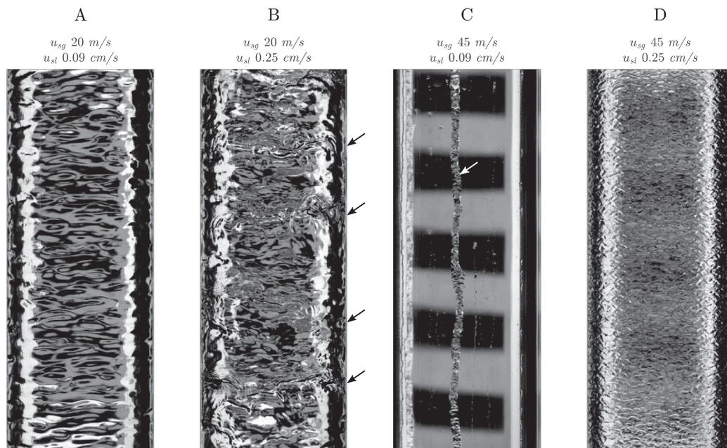
**Fig. 12.** Different film flow regimes observed from the high speed video recordings. (A/D) ripples, (B) ripples and disturbance waves, (C) rivulets. The superficial gas and liquid velocities are indicated on top, in m/s and cm/s, respectively. The black and white bands in the background are used to increase the contrast in the film shadowgraphs. The black arrows indicate the position of disturbance waves in B, whereas the white arrow shows the rivulet observed in C.
