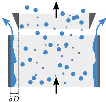
**Fig. 8.** Schematic representation of the slit used to remove the film from the pipe wall.  $\delta D$  indicates the gap width between the inner pipe wall and the slit edge, which is 2 mm at each side.
