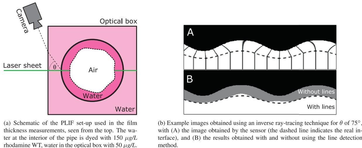
Fig. 5. Principles of the liquid film thickness measurements.
