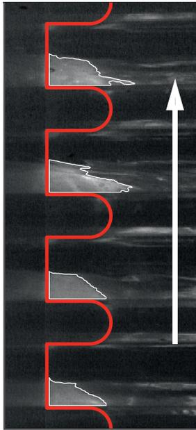
**Fig. 7.** Typical image of liquid accumulation in cavities for a corrugated pipe with geometry B (see Table 1). Flow is from bottom to top. The corrugated wall is marked with the red line, the white boundaries are obtained from image processing and indicate the filling regions. (For interpretation of the references to color in this figure legend, the reader is referred to the web version of this article.)
