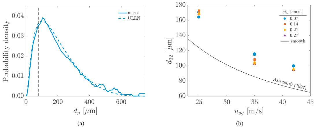
**Fig. 18.** (a) Example of a combined droplet size distribution in the corrugated pipe (geometry A) for  $u_{sg} = 35$  m/s and  $u_{sl} = 0.07$  cm/s, the dashed vertical line indicates the center of the SPI-IPI merging region. (b) Sauter mean diameter of the combined droplet size distributions in a corrugated pipe (geometry A) as a function of superficial gas flow speed. The solid line indicates a correlation for the droplet size in smooth pipes (Azzopardi, 1997).
