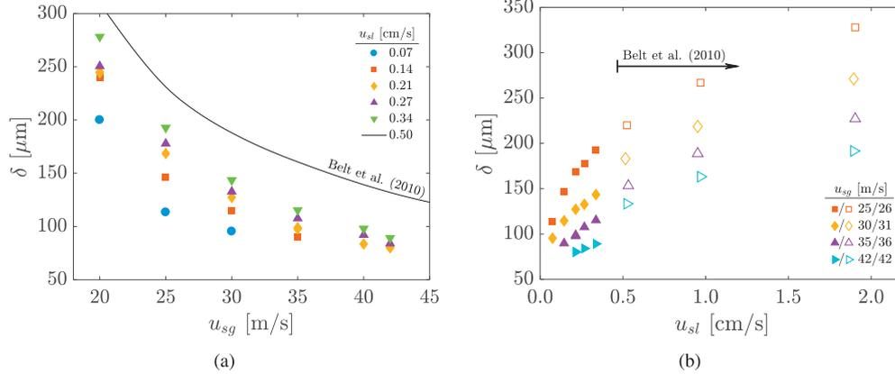
**Fig. 15.** Film thickness ( $\delta$ ) as a function of (a) superficial gas velocity and (b) superficial liquid velocity. The solid line in (a) and open symbols in (b) are experimental data by Belt et al. (2010).
