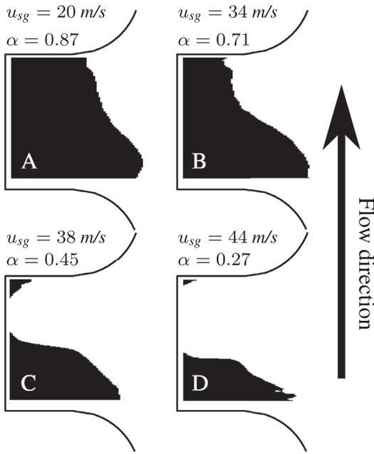
**Fig. 20.** Liquid cavity filling profile, measured with the PLIF method described in Section 2, for the four different cases indicated in Fig. 19a. Flow is from bottom to top and dark regions are regions of liquid accumulation, for  $u_{sl} = 0.11$  cm/s.
