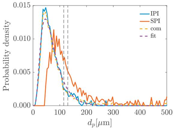
**Fig. 11.** Volumetric droplet size distributions obtained from IPI and SPI, and the resulting combined and fitted distribution. The vertical dashed lines indicate the combination region for this particular case.
