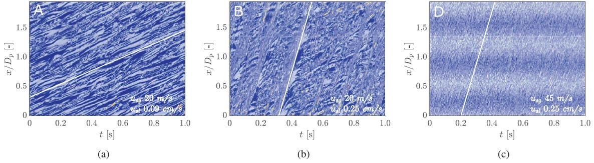
**Fig. 14.** Time-space diagrams of the image intensity along the pipe centerline for  $u_{sg} = 20$  (a,b) and  $45$  m/s (c), and  $u_{sl} = 0.09$  (a) and  $0.25$  cm/s (b,c). The white lines indicate the wave speed of the ripple (a,c) and disturbance (b) waves. The letters in the top left corners correspond to the letters used in Fig. 12.
