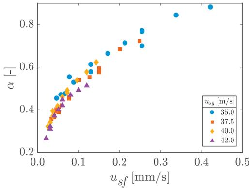
**Fig. 21.** Liquid filling fraction  $\alpha$  as a function of the superficial liquid film velocity ( $u_{sf}$ ) for different values of superficial gas velocity ( $u_{sg}$ ).
