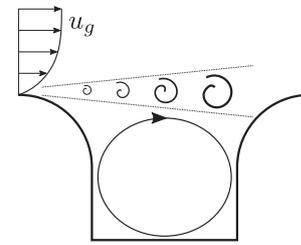
**Fig. 2.** Typical cavity flow in a corrugated pipe, subject to dry gas flow. The incoming gas flow separates at the upstream cavity edge, forming a shear layer where vortical structures can appear. The shear layer separates the bulk flow inside the main pipe from the recirculating flow in the cavities.
