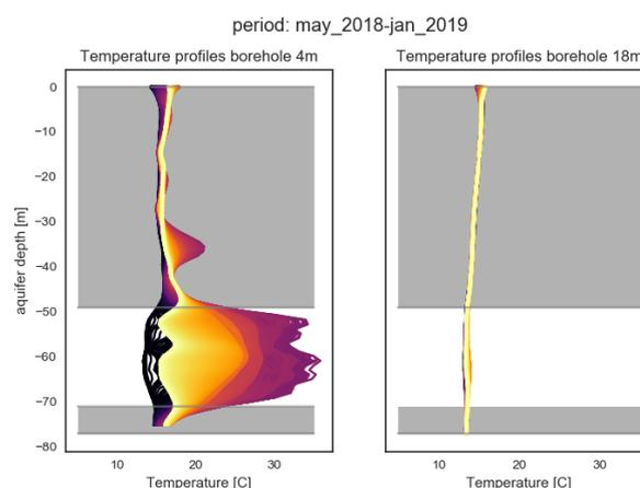
**Figure 3. DTS temperature measurements at warm well, at respectively 4 and 18 m distance. each line is the temperature profile at different time, dark: May '18, light: Jan '19.**
