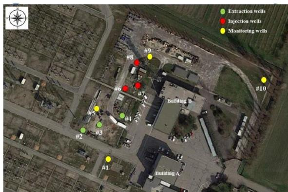
Figure 6: Wells positioning in Bologna pilot site.
