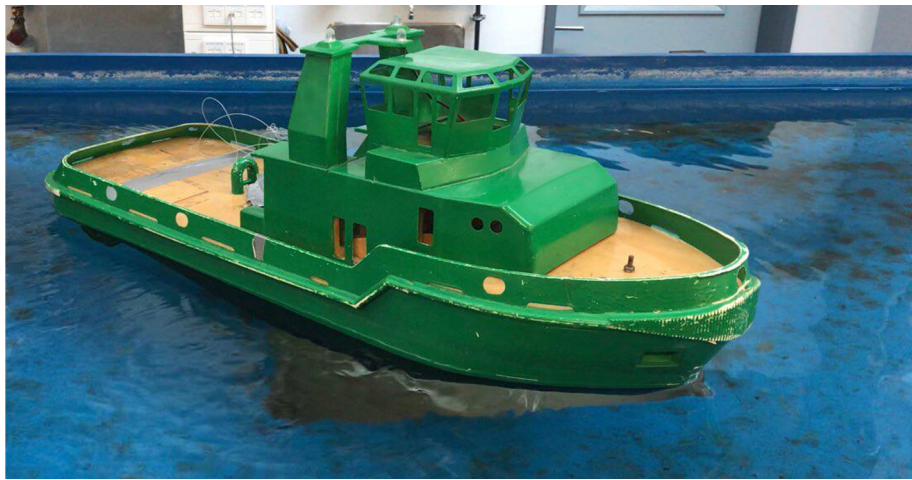
Fig. 5. Tito-Neri: a harbor tug 1:30 replica model [39].
