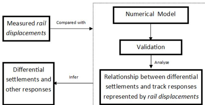
Figure 2. Inspection procedure of track transition zones.
