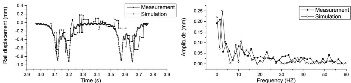
Figure 8. Measured rail displacements of one wagon from train 2 (Figure 5): (a) in time domain and (b) in frequency domain.
