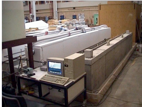
Figure 6.3 View of the test set-up with the thermal isolated beams 1 and 2 and the control-beam 3 in the front, used only for alternate wetting and drying (AWD) (Taheri-Motlagh 1998, Van Breugel 2000).
