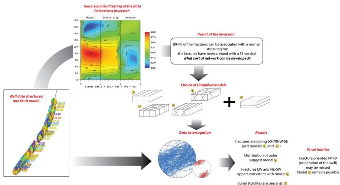
**Figure 2:** method of interpretation and simplification of fracture data coming from wellbore data. This workflow is intended to be used to produce geologically constrained training images to be integrated in the MPS-based workflow
