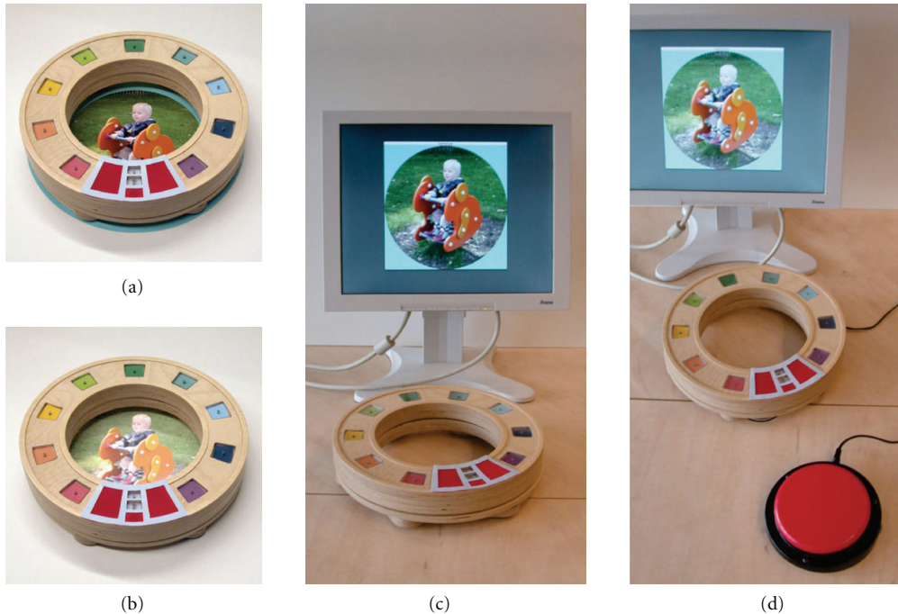
FIGURE 2: The E-Scope in its various configurations: (a) on the floor with pictures (top-left), (b) on a table with an integrated screen (bottom-left, mockup), (c) with a separate screen (middle), and (d) with an additional input device (right).
