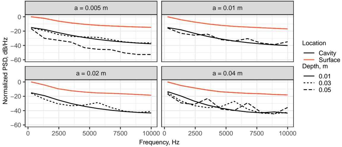
**Fig. 4 Initial model results, velocity = 30 m/sec, modeled acoustic resistance  $R = 2$ , boundary layer modeled with Smol'yakov and Tkachenko model. The four subplots show the results for cavities with radii:  $a = 0.005$  m,  $a = 0.01$  m,  $a = 0.02$  m,  $a = 0.04$  m.**
