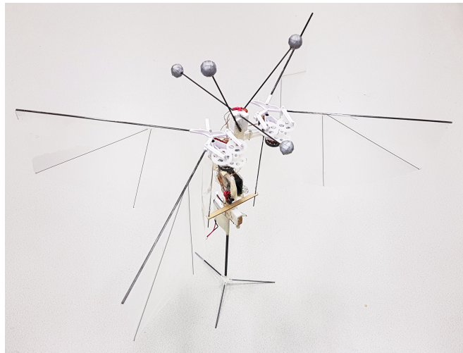
Figure 1: The DelFly Nimble tailless flapping wing robot used for model validation. Its parameters are summarized in Table 1.
