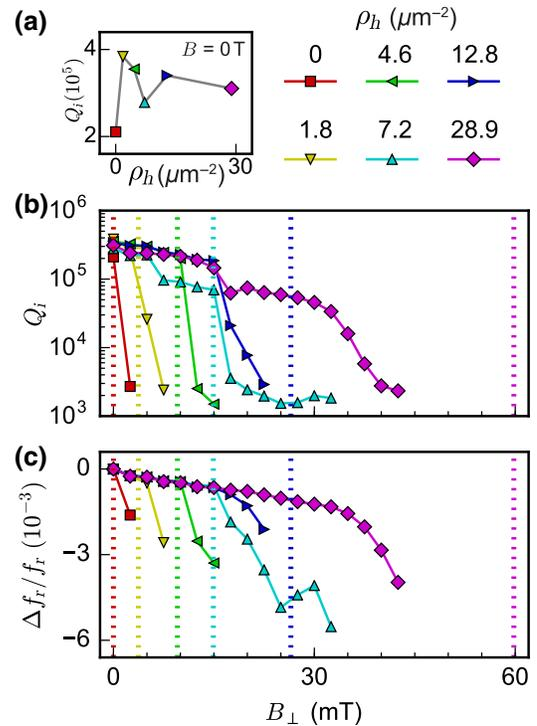
FIG. 3. (a)  $Q_i$  versus  $\rho_h$  for field-cooled resonators at  $B_{\perp} = 0$  T. (b)  $Q_i$  versus  $B_{\perp}$  for varying  $\rho_h$ .  $B_{\text{th}}$  for each resonator is plotted with a color-matched vertical line. (c)  $\Delta f_r/f_r$  versus  $B_{\perp}$  for varying  $\rho_h$  with  $B_{\text{th}}$  plotted as in (b).
