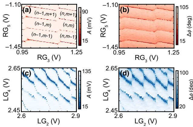
FIG. 6. Measurement of  $S_{21}$  at  $f_r$  at  $B = 1$  T as  $V$  on the fine gates is varied generates charge-stability diagrams of the right (a),(b) and left (c),(d) nanowire DQDs.  $RG_n$  denotes the  $n^{\text{th}}$  gate on the right DQD device. The electron occupation  $n$  ( $m$ ) of the left (right) QD can be modified by tuning the gate voltages.
