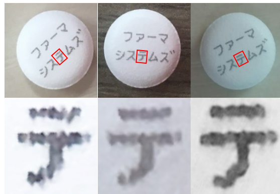
Fig. 4. Tablet images captured using only a smartphone camera (top row). Note that small details of the characters can be captured (bottom row).
