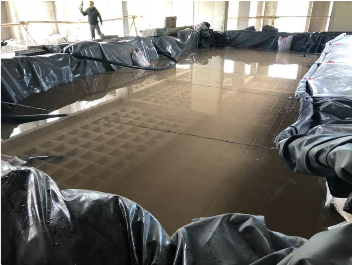
Figure 12. Example of application of dead weight with water. Photograph by S. Camino. Printed with permission.
