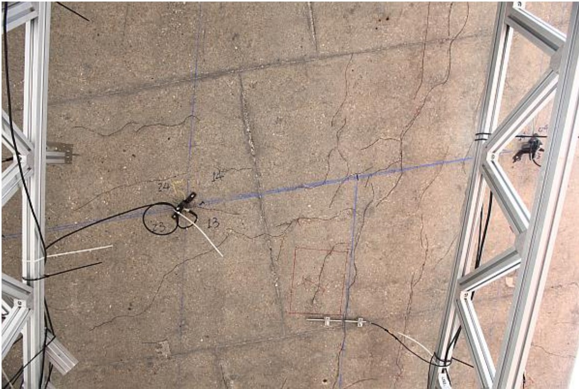
Figure 18. Application of acoustic emissions sensors. Photograph by Y. Yang, used with permission.
