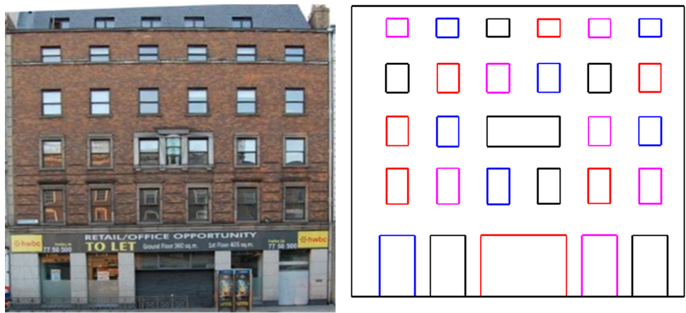
Figure 7: (a) Westmoreland Street Façades and (b) Resulting building reconstruction from the proposed method
