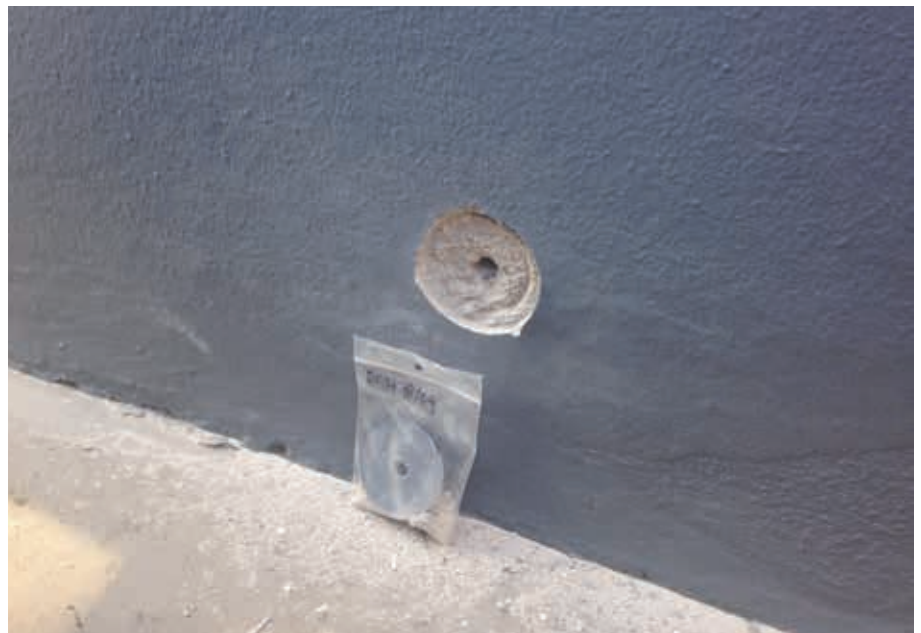
17. In 2018 TNO and Stichting Restauratie Atelier Limburg took samples from specific areas of the exterior and the interior of the Rietveld Schröder House. The photograph shows a sample from the balcony wall on the east elevation (photo author)
