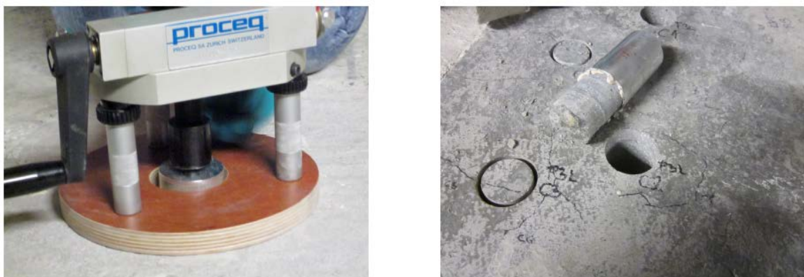
Figure 20: a) Pull-off test set-up and b) Typical failure mode in the substrate
