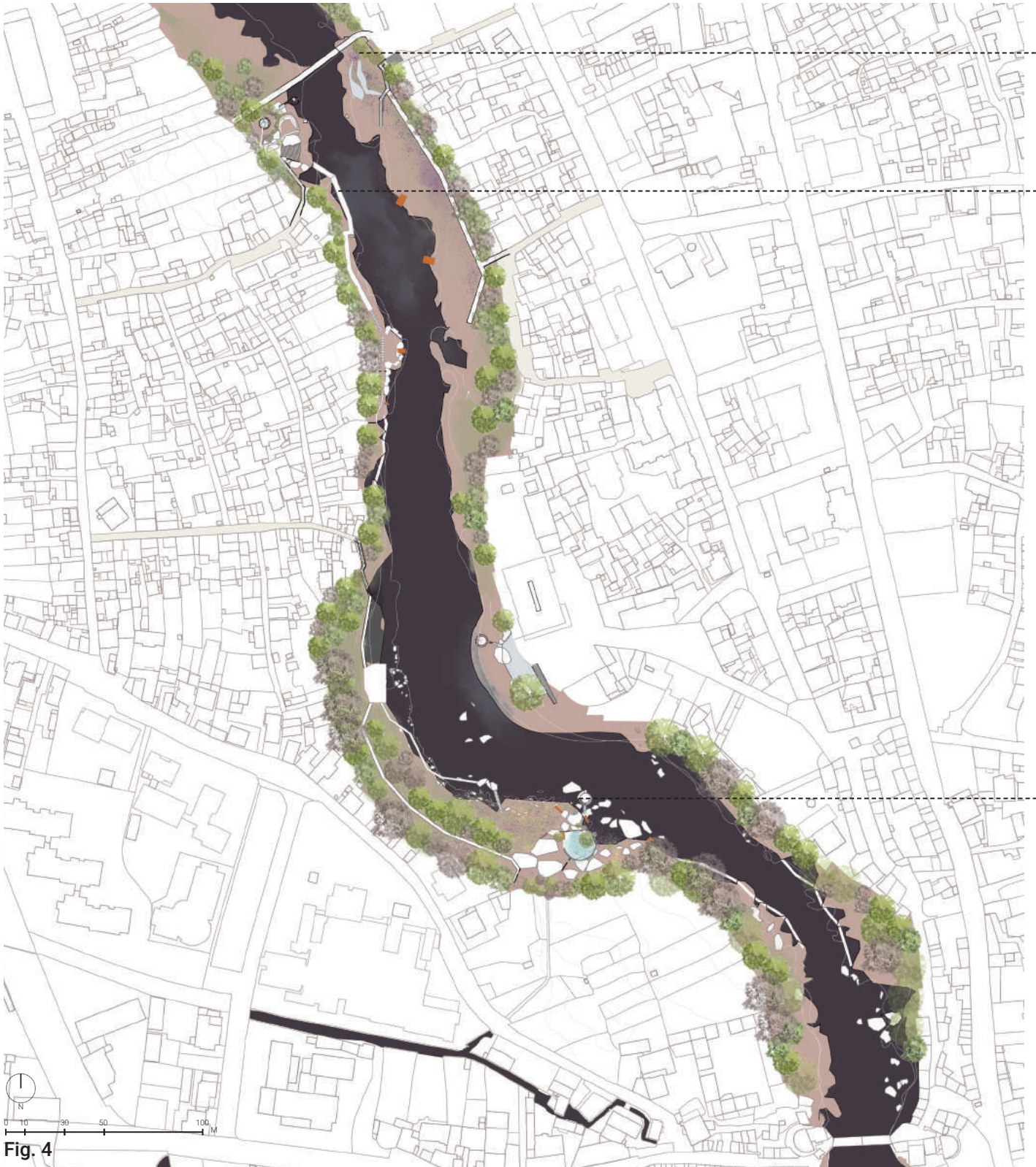
Fig. 3 & 4 explain how the minimal intervention is adapted along the river to enhance the existing landscape affordances and qualities. The impression explains how the river banks adapt to the temporal dynamics of the river. The words for this part were dominance and vulnerability . The left bank responds to erosion by the erosion structures which also work as pathways. On the right, there are two pathways, during high tides they still keep the river bank accessible. These structures also trap sediments and create an environment for hydrophytes. The platforms create smaller territories within this landscape.
