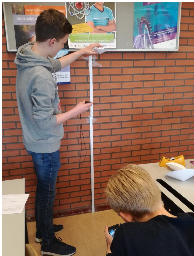
Figure 6. Students drop paper cones with different frontal areas and measure the falling time using both a stopwatch and their mobile phone camera.
