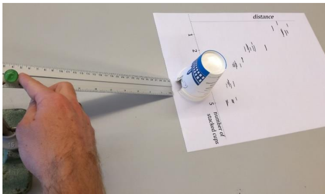
Figure 4. In this activity adopted from Farmer [9], a marble rolls into the stack of cups which then slide across the paper. A line is drawn at that spot. Repeating the procedure reveals variability in the measurements.
