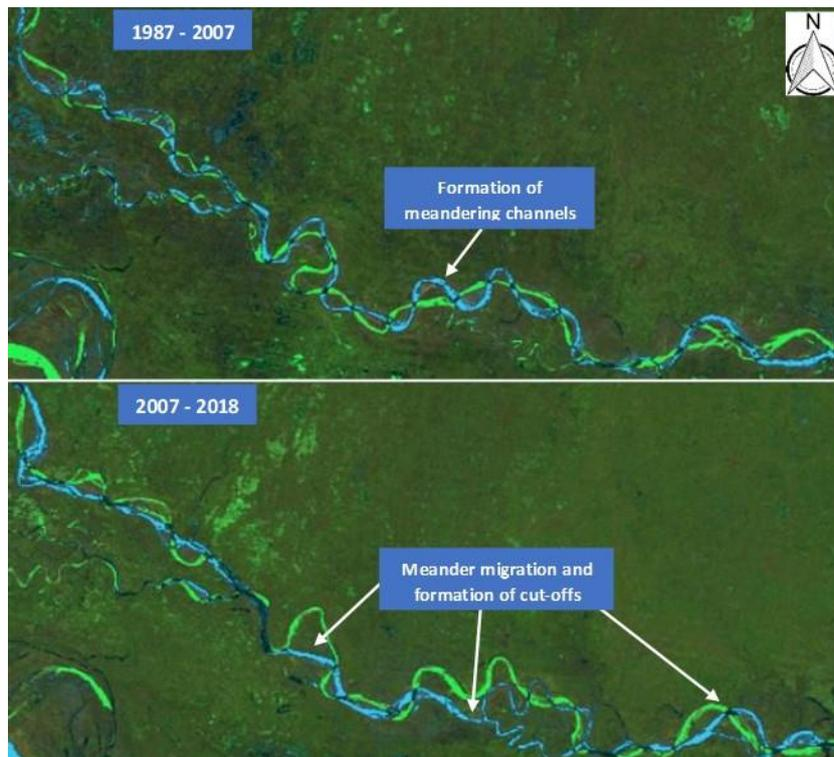
Figure 4. Impacts of upstream changes in flow and sediment transport in downstream reach (in India)
