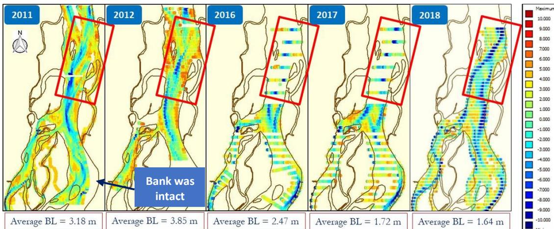
**Figure 8.** Bathymetry measurement, revealing changes in deep-channel patterns upstream of the bifurcation and branches (the average bed level is calculated within the upstream reach indicated by red rectangles, revealing how the reach has become deeper after the intervention)
