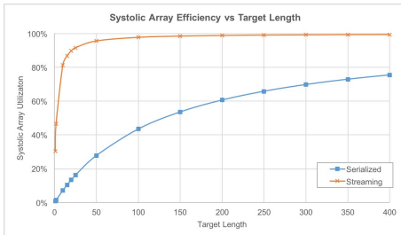
Figure 4. Systolic array efficiency dependence on target length (data set: 100 alignments with query length 131 and variable target length).
