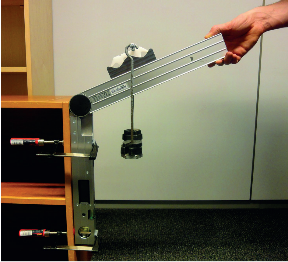
Figure 11. Experimental setup for testing the limits of the range of the application angle. A digital angle measuring device is used to create an inclination table. One leg of the measuring device is clamped to a vertical panel while the other leg can move freely. The bony geometry is fixed onto the inclination table (the free leg). For an experiment the guide is placed onto the bony geometry in the planned position. Weight is hung in one of the grooves of the application surface, representing an application force.
