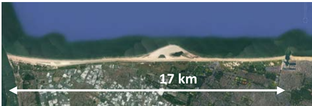
Figure 1, the Sand Engine mega nourishment placed in a 17 km alongshore coastal cell between two harbors.
