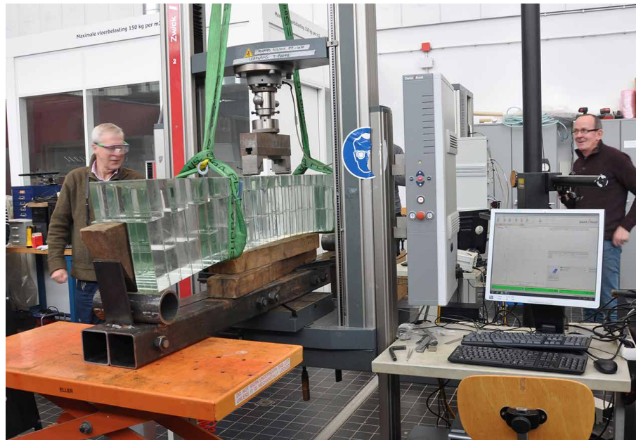
FIG. 5.18 4-point bending set-up of the architrave
