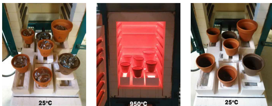
FIG. 7.8 Kiln-casting method employed at the lab for the casting of prototypes.
