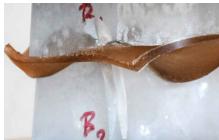
FIG. 8.12 Typical glass failure originating at the edge of the assembly caused by the perforation/tearing of the interlayer (specimen 60A 1 )
