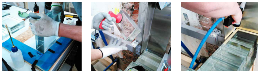
FIG. 6.21 From left to right: Bonding of the steel plate to the corner brick. Positioning of the brick by a suction cup holder. Application of the semi-elastic polymer.
