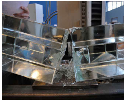
FIG. 5.26 Typical failure mode of specimens, a clear, vertical cut at the middle of the beam.
