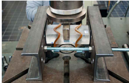
FIG. 8.30 Specimen out of blocks with 15 mm amplitude before testing (top left); at max. deformation (top right); and after failure (bottom left and right).
