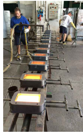
FIG. 2.24 High precision open steel moulds used for the manufacturing of the glass blocks for the Crystal Houses façade.
