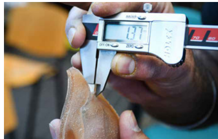
FIG. 8.13 Specimen 60A 3 after the completion of the test. There is evident plastic deformation.
