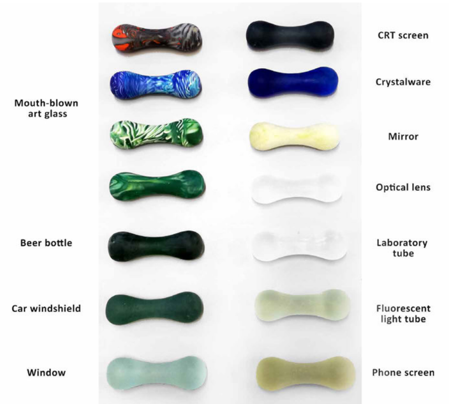
FIG. 7.22 Prototypes of the Type C topology made from the re-melting of different types of glass waste within the context of the Re 3 Glass project.
