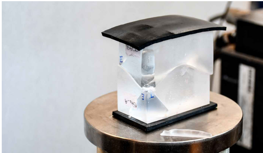
FIG. 8.16 Failure mode of glass specimen without the use of an interlayer.
