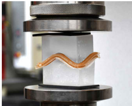
FIG. 8.22 A 6 mm thick 70A specimen, before (left) and during (right) testing under 40 kN constant load.
