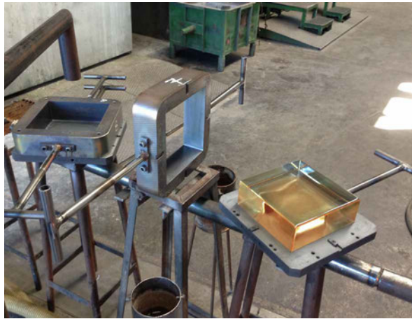
FIG. 2.24 High precision open steel moulds used for the manufacturing of the glass blocks for the Crystal Houses façade.
