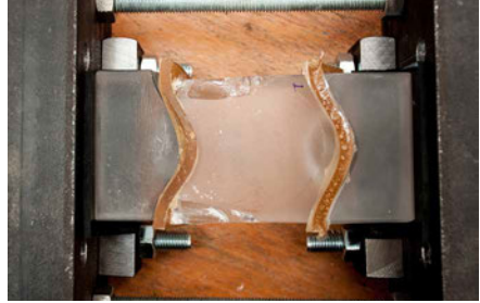
FIG. 8.30 Specimen out of blocks with 15 mm amplitude before testing (top left); at max. deformation (top right); and after failure (bottom left and right).
