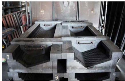
FIG. 2.24 High precision open steel moulds used for the manufacturing of the glass blocks for the Crystal Houses façade.
