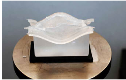
FIG. 8.11 75A specimen after the test was aborted due to visible tearing of the interlayer.
