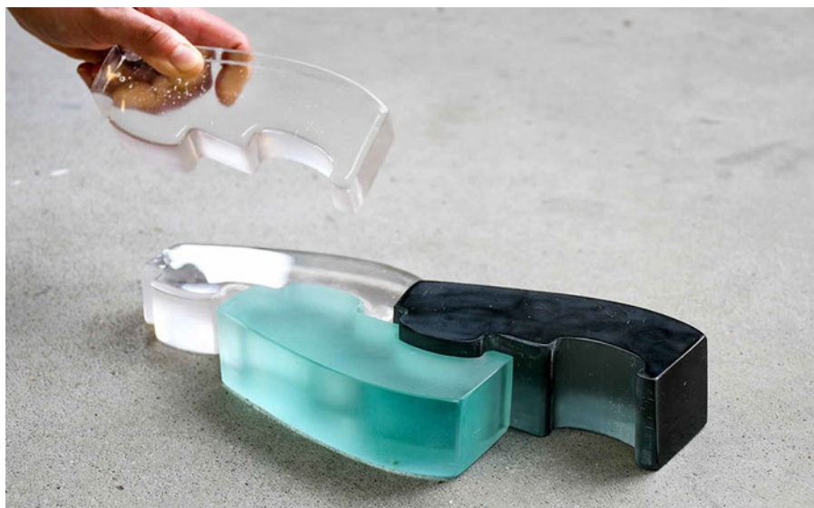
FIG. 7.12 Type D prototype made of clear glass, recycled float glass (teal) and recycled Cathode Ray Tube (CRT) screen (black).
