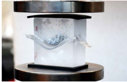
FIG. 8.11 75A specimen after the test was aborted due to visible tearing of the interlayer.
