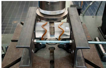
FIG. 8.31 Specimen out of blocks with 20 mm amplitude before testing (top left); at max. deformation (top right); and after failure (bottom left and right)
