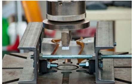
FIG. 8.30 Specimen out of blocks with 15 mm amplitude before testing (top left); at max. deformation (top right); and after failure (bottom left and right).
