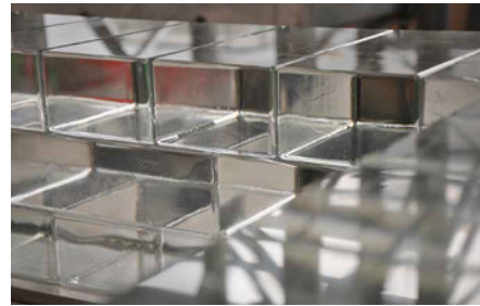
FIG. 6.15 Left: Sealing of the already bonded bricks. Right: the final, visual result achieved by the novel bonding method.
