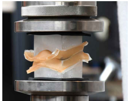
FIG. 8.22 A 6 mm thick 70A specimen, before (left) and during (right) testing under 40 kN constant load.
