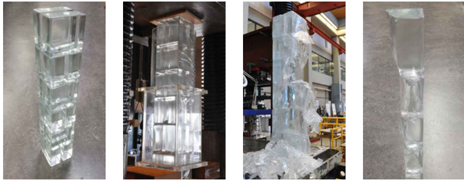
FIG. 5.23 Left: B_{NS} column prior to testing. Centre left: Initiation of crack. Centre right: Same specimen at complete failure. Right: Intact piece of the tested specimen after failure: the principal crack essentially propagated vertically, defying the adhesive joints.
