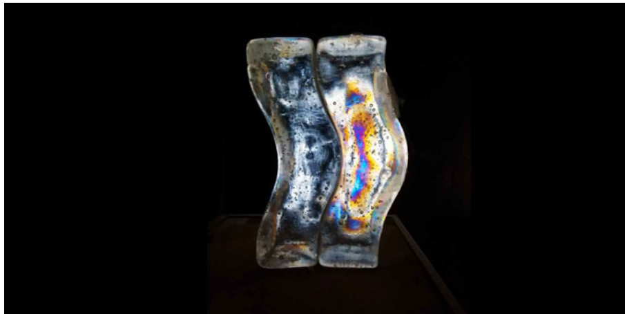
FIG. 2.21 Qualitative analysis of strain concentration by polarization test. Bricks such as the ones shown on the right have a clear indication of residual stresses. Elements with grey-scale spectral composition, such as the one on the left, have low residual stresses.
