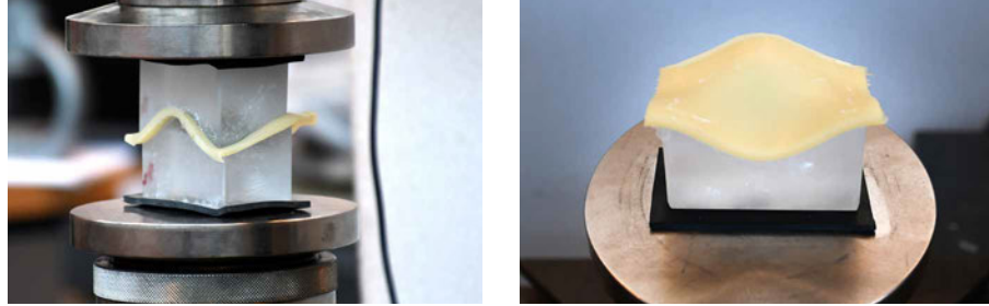
FIG. 8.14 One of the 80A interlayer specimens during (right) and after (left) testing. No visible plastic deformation was observed.
