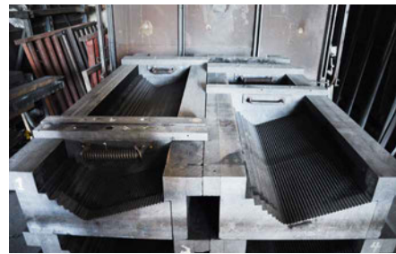
FIG. 2.24 High precision open steel moulds used for the manufacturing of the glass blocks for the Crystal Houses façade.
