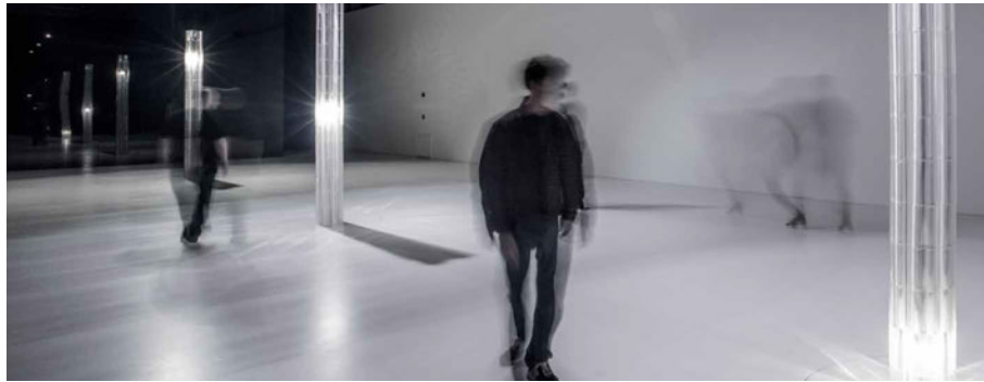
FIG. 2.13 3m tall glass prototypes out of 3D-printed segments. Source: Paula Aguilera, Jonathan Williams and The Mediated Matter Group.
