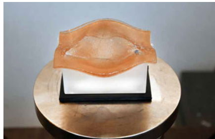
FIG. 8.13 Specimen 60A 3 after the completion of the test. There is evident plastic deformation.
