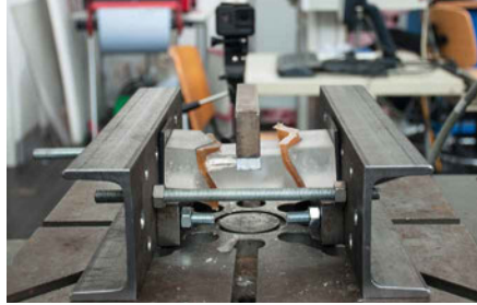
FIG. 8.30 Specimen out of blocks with 15 mm amplitude before testing (top left); at max. deformation (top right); and after failure (bottom left and right).
