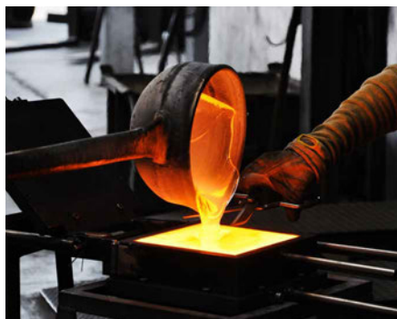
FIG. 2.16 Left: Primary casting method (hot-forming). Right: Secondary casting method (kiln-casting).
