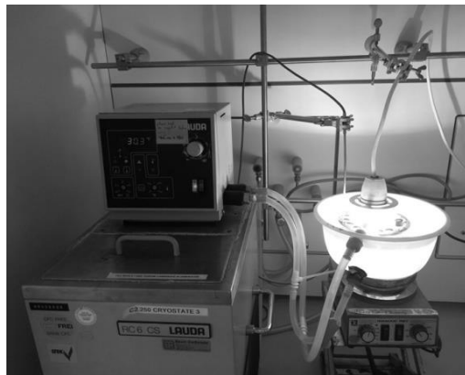
Figure 15. Reaction setups used for the photo-chemical reactions. Left: the temperature controlled reaction setup with the incandescent white light bulb. Reaction vials were put in the holder around the light source. Right: reaction setup with the Hamamatsu spotlight at room temperature. Reactions were performed in a closed off, cut off 50 ml falcon tube in order to minimize evaporation.
