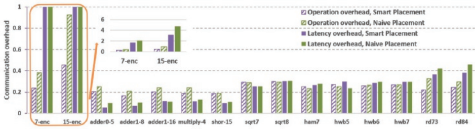
Figure 4.22: Comparison of mapping FT circuits with different initial placements on the checkerboard architecture ( d = 7 ).
