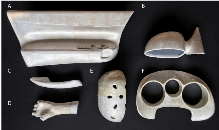
**Figure 1: Examples of delignified densified wood composite parts.** (A) Door panel, (B) side mirror, (C) door handle of a car, (D) orthosis, (E) cut open helmet, and (F) tachometer cover of a car. [Please click here to view a larger version of this figure.](#)
