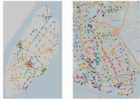
Fig. 1: The medium voltage networks of Texel (left) and Zaan-dam (right). The distribution networks have 226 buses and 406 buses respectively.
