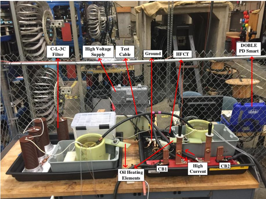
Figure A.3: Experimental set-up for PD measurements in test cables under AC and DC voltages.
