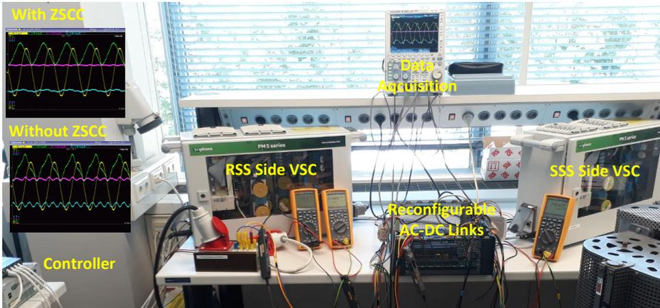
Figure 4.17: Test Setup used to validate key control concepts.
